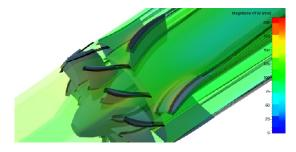
All mechanical components of the fan have been designed with a special focus on durability and robustness. For example the 35mm hollow shaft from aluminum 7075 provides highest stiffness. Such mechanical feature allows for a fan composition with minimum blade clearance.
